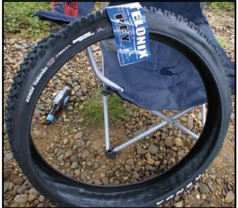
The tire's thread is one of the most aggressive patterns I have seen on a mountain bike tire. Large pronounced center knobs broken down into two staggered positions that reach out towards the mid-point of the tire's crown. The side knobs are also pronounced with a square "H" type shape that is also in a staggered pattern. Right off the bat this is not going to be a fast rolling tire, rather the claim to fame for this tire is its insane traction on varying trail conditions and terrain.
